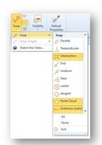
The Object Snaps bind a representative point of the object that you are drawing (e.g. the ending node of a vertical envelope) at a certain point of another object (e.g. at the edge or midpoint of a column, etc.).
